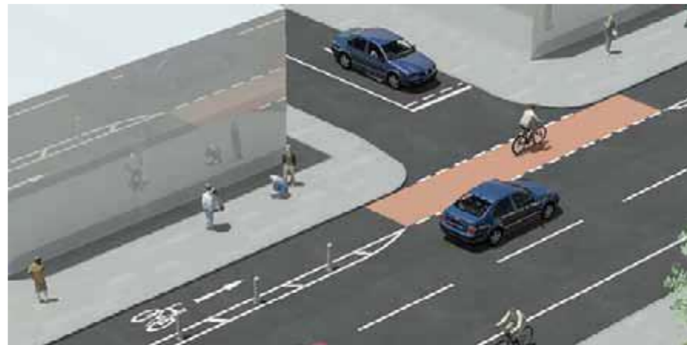
Figure 32: On-Road Cycle Lane Priority Junction Treatment
