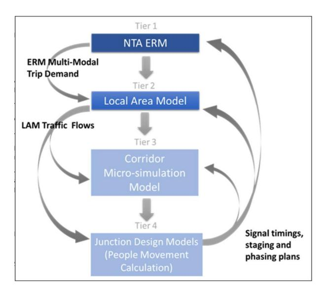
Figure 2-1 Transport Modelling Methodology and Information Flow
