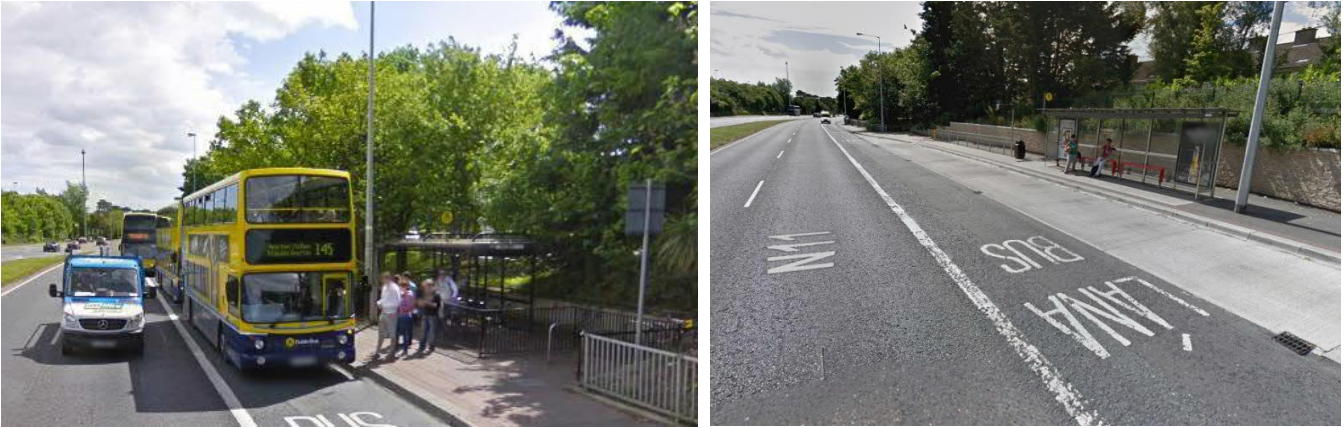
Figure 1.5 Stillorgan QBC with high bus flows and no bus laybys resulted in bus bunching/ platooning; bus lay-by's provided at key locations to allow express buses to pass slower buses. (Source: Google Maps)
