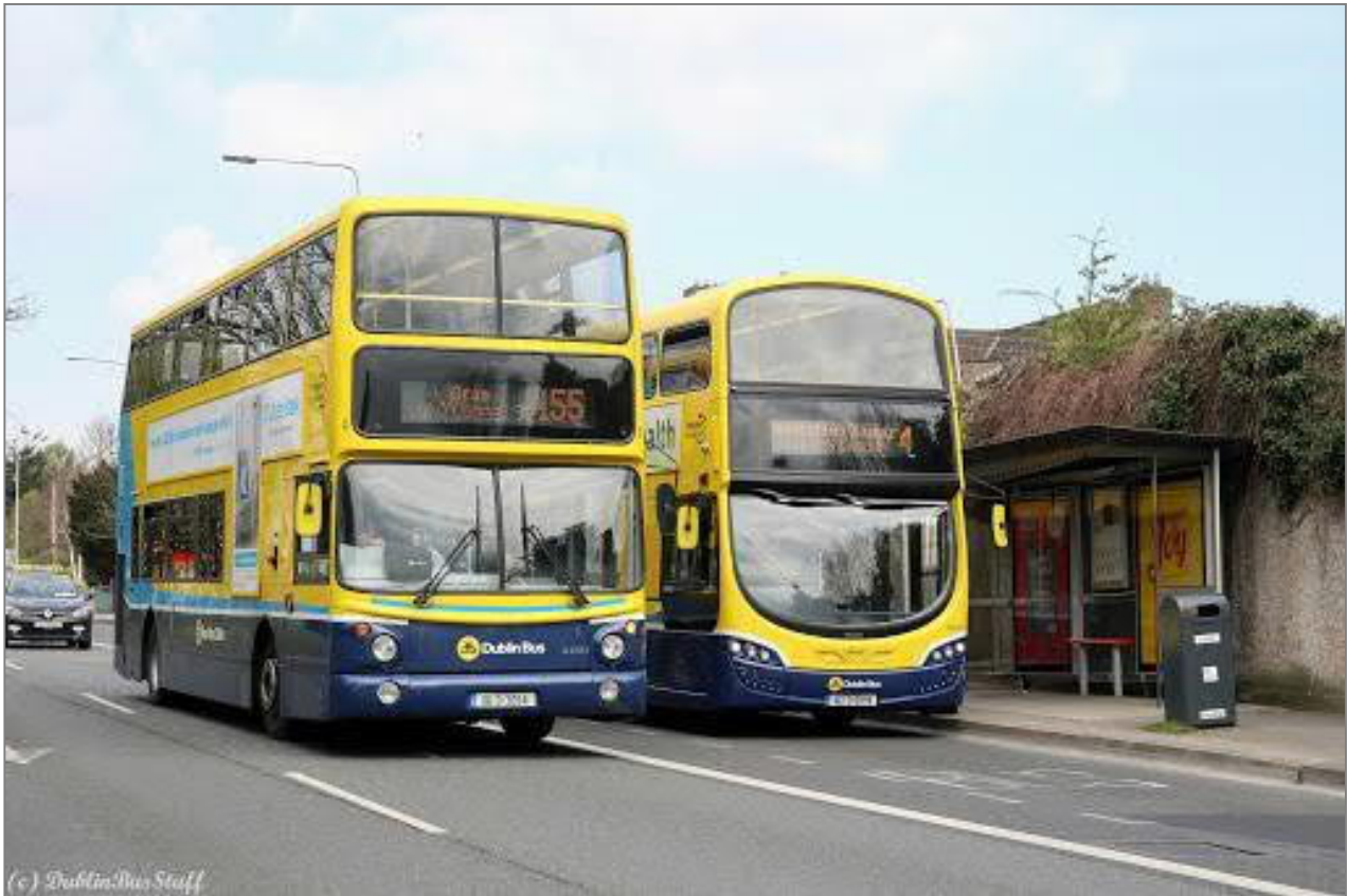
Figure 7.3 In-line bus stops on a heavily used bus corridor can lead to express, or non-stopping buses, being delayed or making overtaking manoeuvres. (source: Dublin Bus Stuff).
