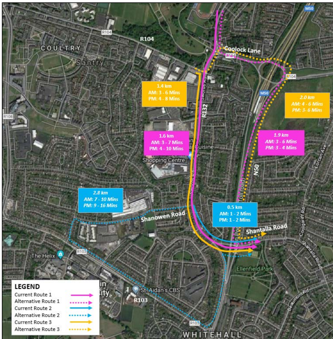
Figure 5.14: Alternative Routes Available for Traffic Originating North or West of Santry with a Destination on Shantalla Road
