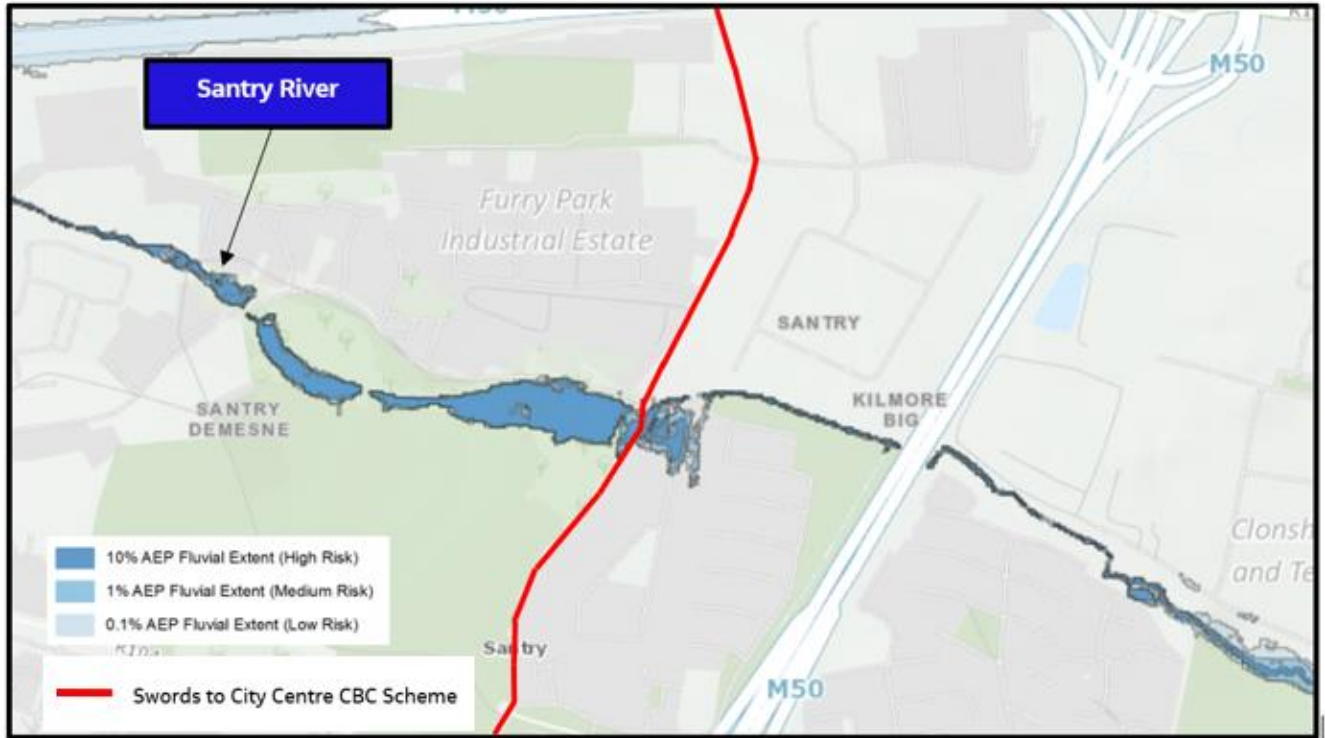
Figure 4.9 Extract of Fluvial flood mapping from Eastern CFRAM study for the Scheme 2 at the crossing with Santry River.
