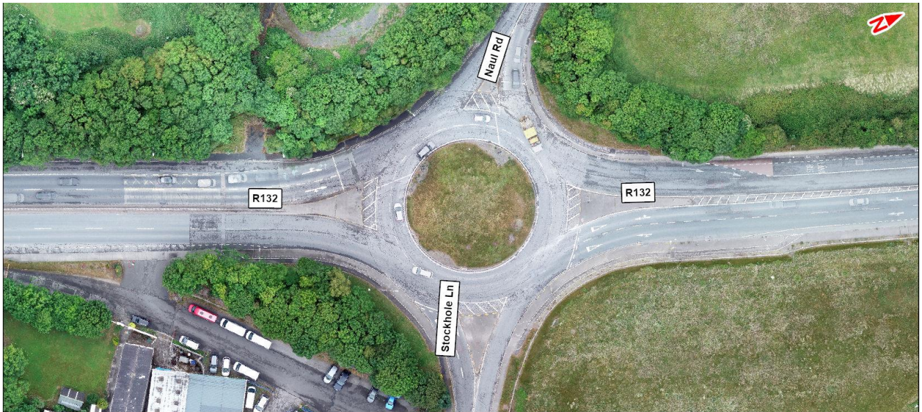
Image 6.4: Cloghran Roundabout Arrangement
