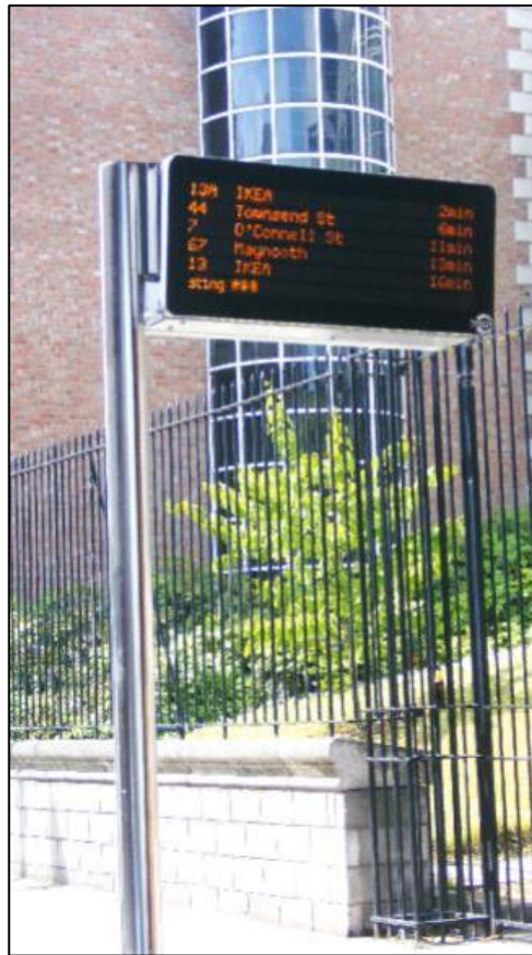
Figure 12.1: RTPI Display at Bus Stop
