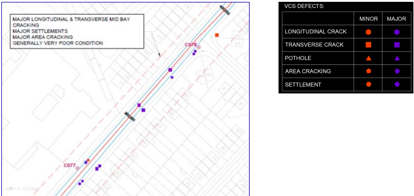
Figure 7.1: Example Ranking of Pavement Condition and the Type and Location of Defects Observed.
